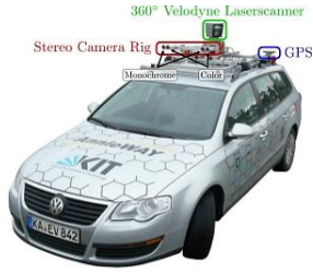
Fig. 5. The KITTI database we use for our experiments is recorded from a moving car equipped with several cameras, a GPS device and most notably a Velodyne LIDAR device.
